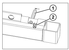
Fig. 8-16: Pulling out the locking lever
