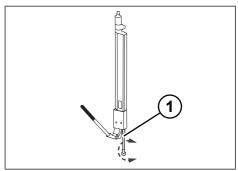
Fig. 6-50: Closing the drain valve
