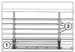
Fig. 6-44: Load compartment limiter with board walls and plug-in laths
