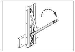
Fig. 6-33: Folding down the locking lever
