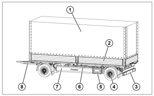
Fig. 3-4: Turnframe trailer (2-axle) with full-tarp superstructure
