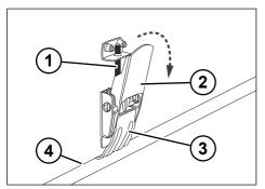
Fig. 6-18: Releasing the direct tensioner
