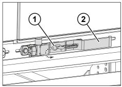
Fig. 6-4: Door lock with two-handed operation
