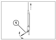
Fig. 6-51: Raising the lifting roof
