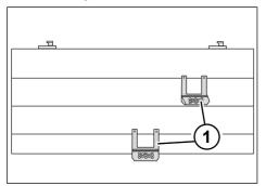
Fig. 5-34: Fold-down steps on the folding rear wall
