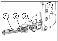
Fig. 6-23: Rear curtain tensioning device
