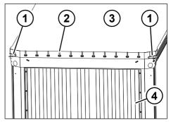
Fig. 6-47: Sliding roof on the front wall side
