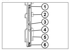
Fig. 6-31: Telescopic fold-out post
