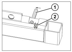
Fig. 8-13: Pulling out the locking lever
