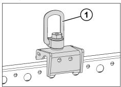
Fig. 8-10: Multi Flex Flat chain adapter
