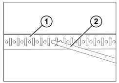
Fig. 8-5: Attach the telescopic lock rod
