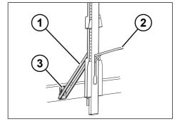
Fig. 6-30: Releasing the one-part fold-out post
