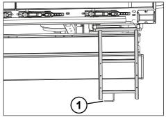
Fig. 5-33: Folding telescopic ladder in the function position
