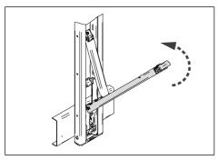
Fig. 6-35: Closing the locking lever
