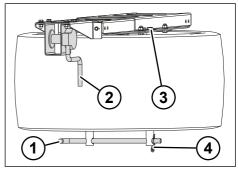
Fig. 5-37: Spare wheel with winch
