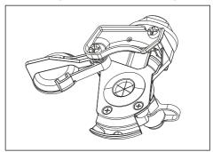
Fig. 5-14: Example of standard coupling head
