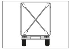
Fig. 7-4: Cross-bracing of the rear gantry
