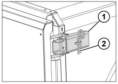
Fig. 5-41: Tension lock
