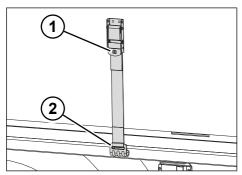
Fig. 6-16: Anti-tilt curtain buckle
