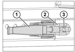
Fig. 8-21: Lock lever secured on the footing beam
