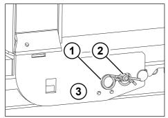
Fig. 8-22: Sliding shoe secured with plug-in bolt and spring cotter pin
