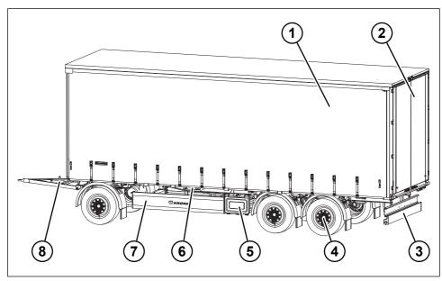
Fig. 3-3: Turnframe trailer (3-axle) with sliding curtain superstructure
