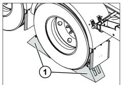
Fig. 5-1: Putting on the wheel chocks
