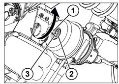
Fig. 5-25: Deactivating the emergency release screw
