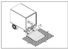
Fig. 6-13: Hazard area of the tail lift
