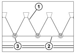
Fig. 6-19: Attached rubber expanders
