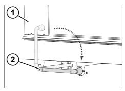
Fig. 6-8: Swivelling the door stop downwards
