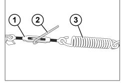
Fig. 5-7: Tension spring with turnbuckle
