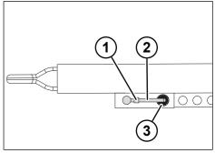
Fig. 5-10: Length adjustment via rapid resetting
