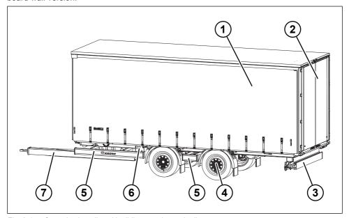
Fig. 3-1: Central axle trailer with sliding curtain semitrailer
