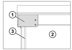
Fig. 6-22: Thread the channel rail
