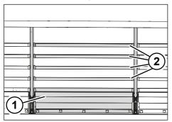
Fig. 6-25: Load compartment limiter with board walls and plug-in laths
