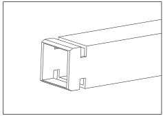
Fig. 8-17: Recesses on the Multi Wall transverse beam
