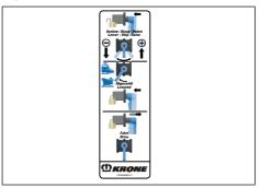
Fig. 5-26: Example pictogram of mechanically controlled air suspension
