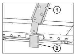
Fig. 6-40: Lifting out the tilting/plug-in post
