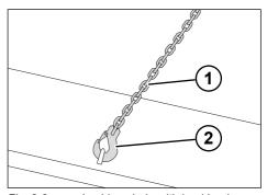
Fig. 8-2: Lashing chain with load hook
