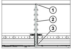
Fig. 6-39: Tilting/plug-in post
