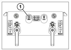
Fig. 5-22: Parking brake for turnframe trailer
