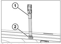
Fig. 6-15: Latch-type curtain buckle
