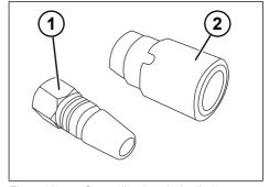
Fig. 5-16: C-coupling heads (trailer)
