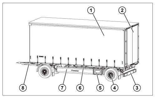
Fig. 3-2: Turnframe trailer (2-axle) with sliding curtain superstructure
