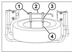
Fig. 5-38: Spare wheel bracket for twin and tractor vehicle tyres
