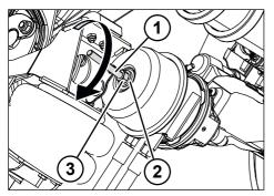
Fig. 5-24: Activating the emergency release screw
