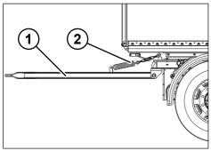
Fig. 5-6: Draw fork with height adjustment device
