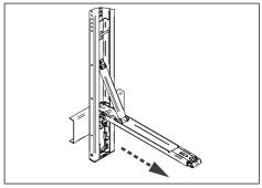
Fig. 6-34: Swivelling the post away from the vehicle
