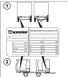
Fig. 1-1: Type plate attachment points
