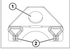
Fig. 8-9: Multi Flex chain adapter
