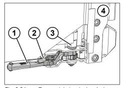
Fig. 6-24: Rear curtain tensioning device
