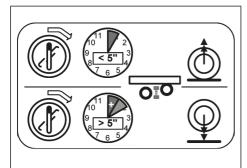
Fig. 5-30: Control switch functions of the lift axle control system
