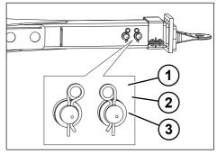
Fig. 5-11: Plug-in bolts on drawbar wale
