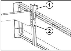
Fig. 5-35: Folded-down side collision protection ((rear view))
