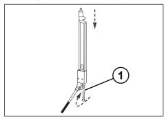
Fig. 6-52: Lowering the lifting roof
