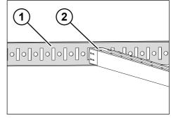
Fig. 8-4: Load securing rails with telescopic lock bars
