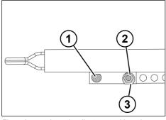
Fig. 5-9: Length adjustment with tool
