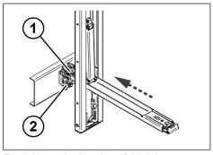
Fig. 6-36: Locking lever folded down
