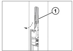
Fig. 6-53: Swivelling the adjustment bolt outwards
