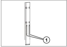
Fig. 6-1: Post with integrated board wall locks
