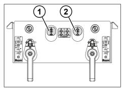
Fig. 7-3: Control unit for brake system of turnframe trailer
