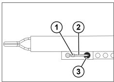
Fig. 5-10: Length adjustment via rapid resetting
