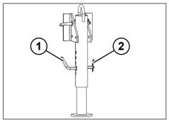
Fig. 5-5: Adjusting the height of the rear brace
