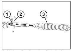
*Fig. 5-8:* Tension spring with turnbuckle, version 2
