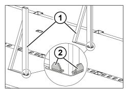
Fig. 6-9: Bracket on plug-in post
