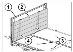
Fig. 6-7: Mobile front wall in the foremost position
