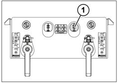
*Fig. 5-20:* Service brake for the turnframe trailer
