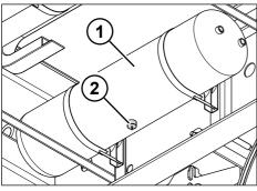
Fig. 5-18: Compressed air tank
