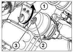
Fig. 5-25: Deactivating the emergency release screw
