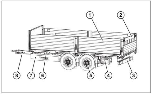
Fig. 3-2: Overview of the central axle version of the Load Carrier building material trailer
