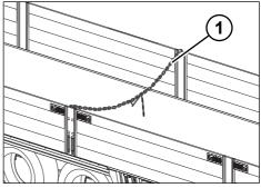
Fig. 8-4: Using tension chains
