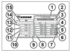
Fig. 1-2: Example type plate
