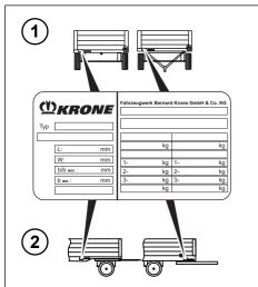
Fig. 1-1: Type plate attachment points
