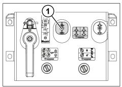
Fig. 5-21: Parking brake for central axle trailer
