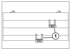
Fig. 5-32: Fold-down steps on the folding rear wall
