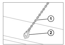
*Fig.* 8-2: Lashing chain with load hook
