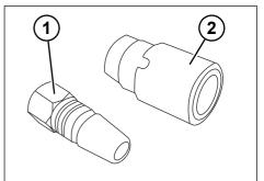
Fig. 5-16: C-coupling heads (trailer)
