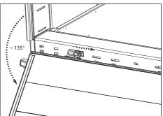
Fig. 6-5: Folding down the rear wall
