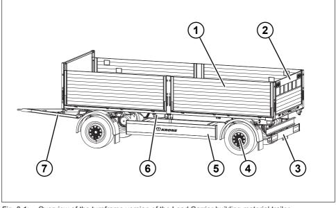
Fig. 3-1: Overview of the turnframe version of the Load Carrier building material trailer
