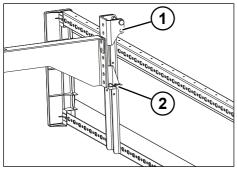
*Fig. 5-33:* Folded-down side collision protection ((rear view))
