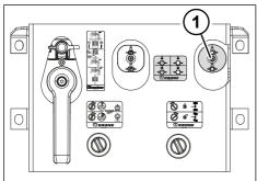
*Fig. 5-19:* Service brake for the central axle trailer
