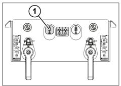
Fig. 5-22: Parking brake for turnframe trailer
