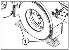
*Fig. 5-1:* Putting on the wheel chocks
