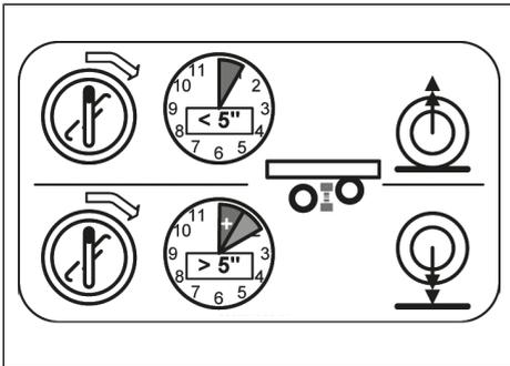
Fig. 5-30: Control switch functions of the lift axle control system
