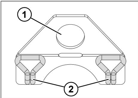
Fig. 8-8: Multi Flex chain adapter
