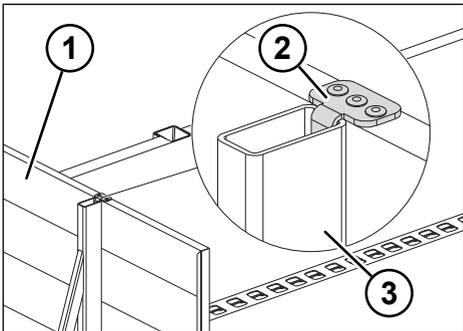
Fig. 6-8: Mobile front wall fastening hooks
