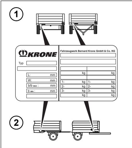
Fig. 1-1: Type plate attachment points
