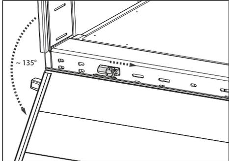
Fig. 6-5: Folding down the rear wall
