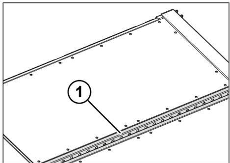
Fig. 8-15: Multi Rail lashing rail
