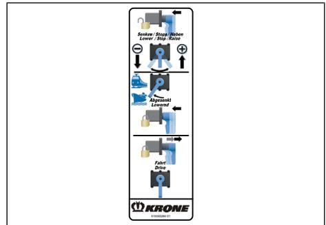
Fig. 5-26: Example pictogram of mechanically controlled air suspension
