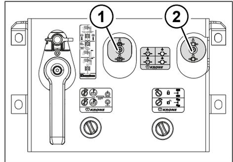
Fig. 7-2: Control unit for brake system of central axle trailer
