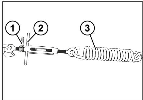
Fig. 5-8: Tension spring with turnbuckle, version 2
