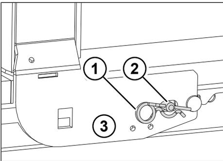
Fig. 8-14: Sliding shoe secured with plug-in bolt and spring cotter pin
