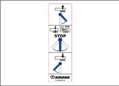
Fig. 5-27: Example pictogram of electronically controlled air suspension
