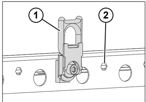
Fig. 8-6: Multi Lash with Multilock external frame
