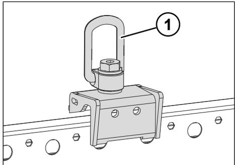
Fig. 8-9: Multi Flex Flat chain adapter
