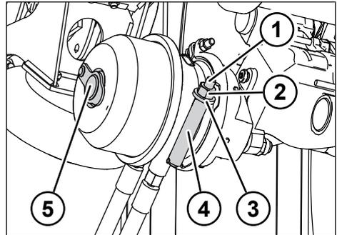
Fig. 5-23: Spring storage with emergency release device
