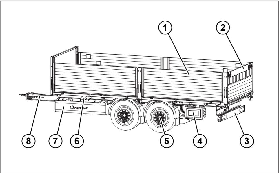
Fig. 3-2: Overview of the central axle version of the Load Carrier building material trailer
