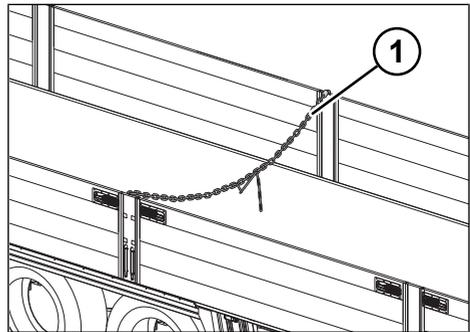
Fig. 8-4: Using tension chains
