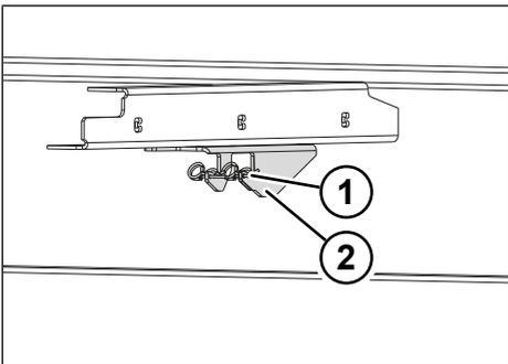
Fig. 5-40: Bracket for Multi Block beams
