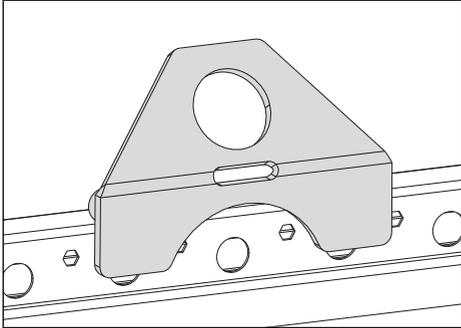
Fig. 8-7: Multi Flex chain adapter with Multilock external frame
