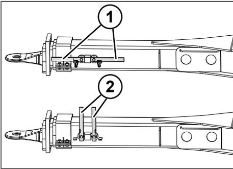
Fig. 5-12: Hand lever on the drawbar wale
