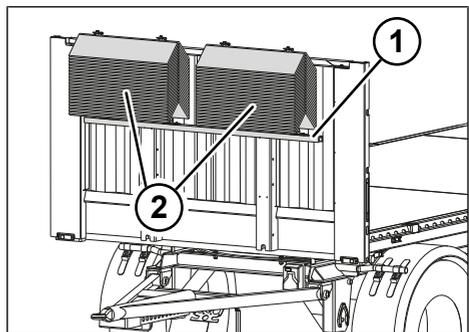
Fig. 6-10: Front wall depot for edge protectors
