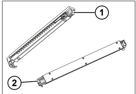
Fig. 8-12: Multi Fix footing beam
