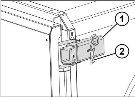
Fig. 5-38: Tension lock
