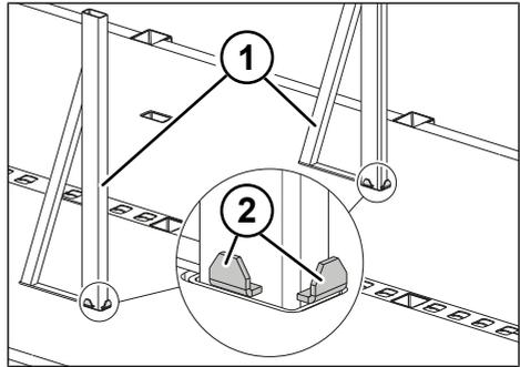
Fig. 6-9: Bracket on plug-in post
