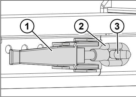
Fig. 8-13: Lock lever secured on the footing beam
