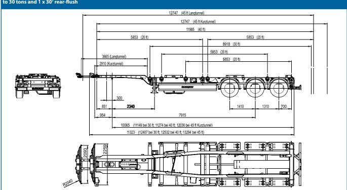
Attention: Transport of filled tank container is not allowed! Container position 20' in centre position limited to 30 tons. During transport of 45' containers with short tunnel the allowed length from the king pin to the rear is exceeding legal limits! The transport of 45' containers with long tunnel and chamfered corners at front is possible within the EC directive. The rear bumper must be pulled out manually!
