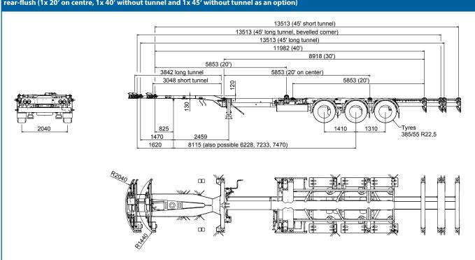
Attention: Transport of filled tank container is not allowed! The transport of 45' containers with long tunnel and chamfered corners at front is possible within the EC directive (while using the optional front extension). During transport of 45' containers with short tunnel the allowed length from the king pin to the rear is exceeding legal limits!
