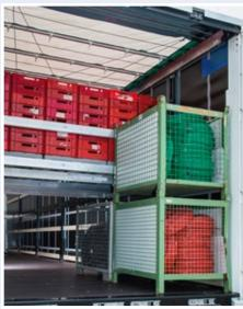
The double deck includes 12 side double bars with an integrated lock rail for side to side. 23 side to side double deck bars are included. This results 33 pallet storage spaces in the second level with the capacity of max. 320 kg per pallet.
