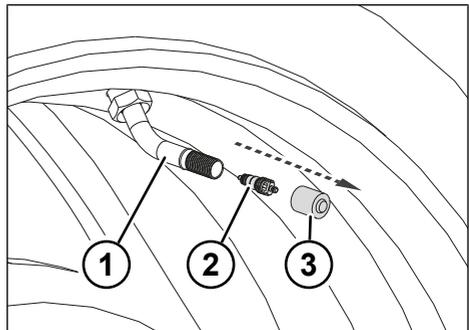
Fig. 4-9: Removing the valve insert
