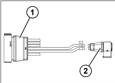
Fig. 4-14: KSC wiring harness
