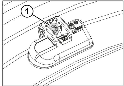
Fig. 4-5: Tightening the screws
