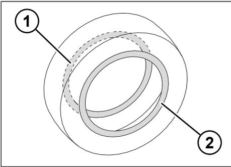
Fig. 4-7: Applying assembly paste
