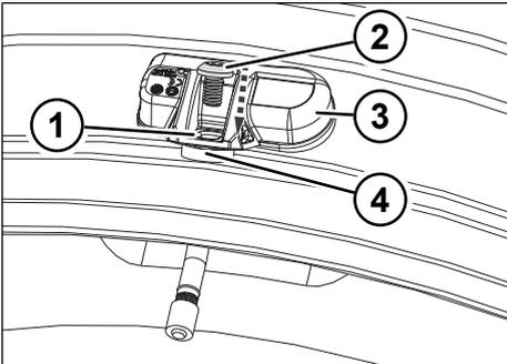
Fig. 4-4: Screwing the screw in the valve thread
