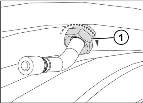
Fig. 4-3: Tightening the union nut
