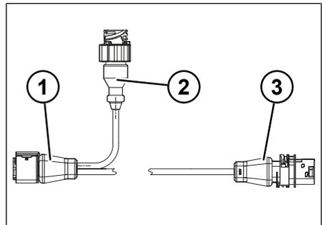
Fig. 4-13: KRONE Smart Tyre Monitoring System wiring harness
