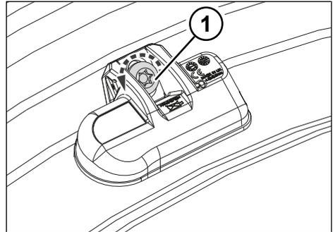
Fig. 7-4: Removing the screw
