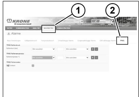
Fig. 6-2: Defining the warning signals (screenshot of the KRONE Telematics Portal)
