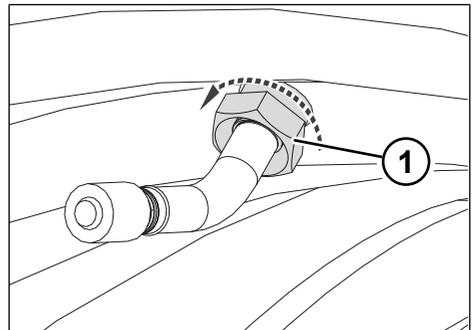
Fig. 7-5: Removing the union nut
