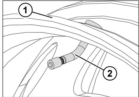
Fig. 4-1: Inserting the valve in the rim
