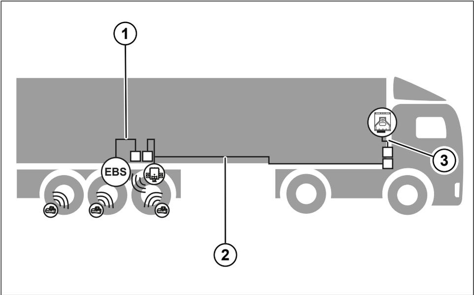
Fig. 4-12: Cable routing
