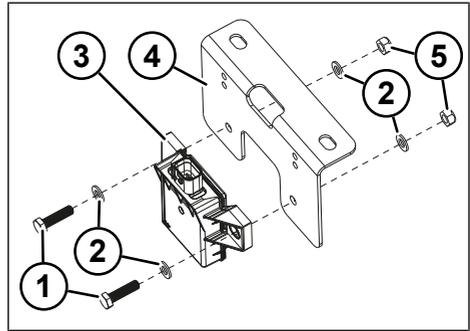
Fig. 7-8: Dismounting the control unit
