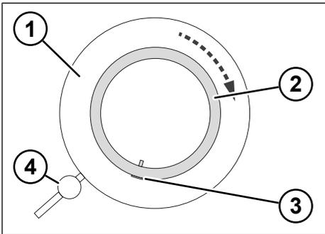
Fig. 7-3: Disassembly of the bottom tyre bead
