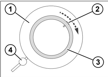
Fig. 4-8: Installation of the bottom tyre bead
