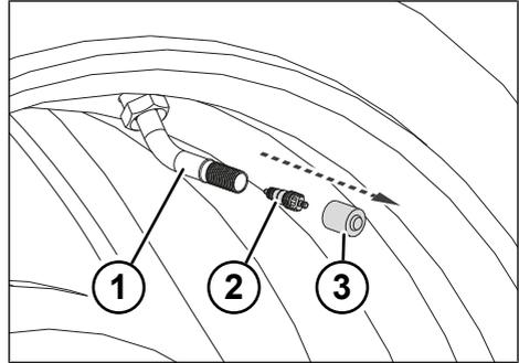
Fig. 7-1: Removing the valve insert
