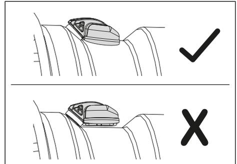
Fig. 4-6: Wheel sensor position
