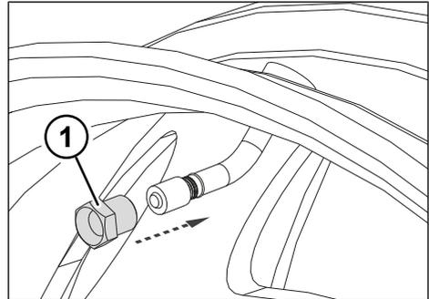
Fig. 4-2: Slide the union nut onto the valve
