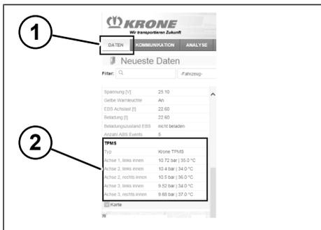
Fig. 6-1: Smart Tyre Monitoring System data (screenshot of the KRONE Telematics Portal)
