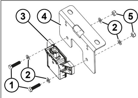
Fig. 4-10: Installation of the control unit
