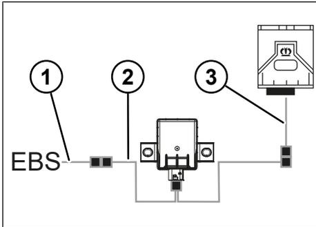
Fig. 3-4: Basic principle Smart Tyre Monitoring System cabling
