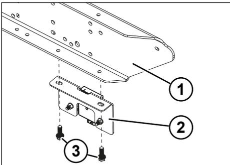
Fig. 7-7: Removing the bracket
