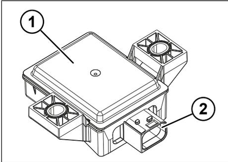
Fig. 3-2: Electronic control unit
